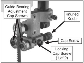
Figure 33. Blade guide bearing controls.
